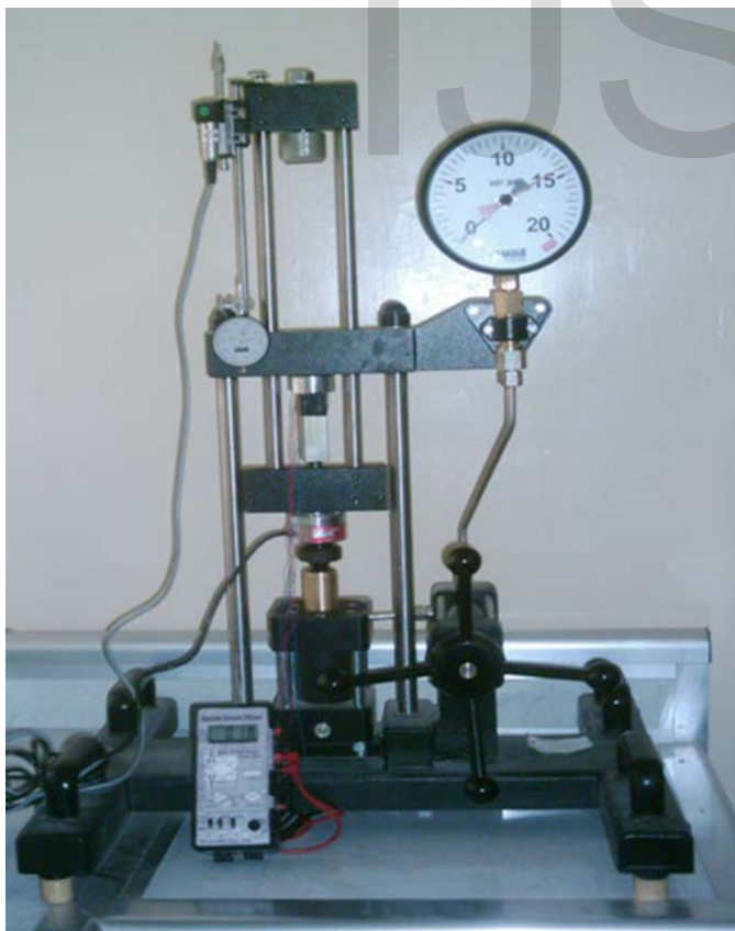
Fig.5. Universal Testing Machine with load cell and strain meter.
